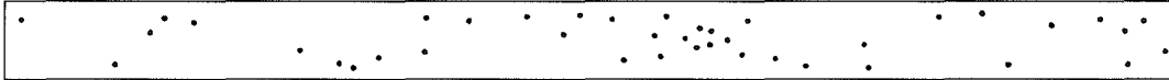
Typical Quantity and Size Permitted in 6 in. (150 mm) Length of Weld \frac{1}{8} in. (3 mm) to \frac{1}{4} in. (6 mm) Thickness
