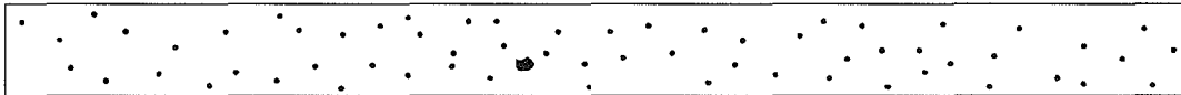
Typical Quantity and Size Permitted in 6 in. (150 mm) Length of Weld Over \frac{1}{4} in. (6 mm) to \frac{1}{2} in. (13 mm) Thickness
